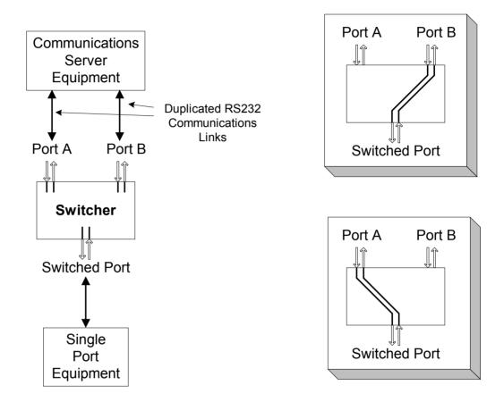
The role of the switch is to monitor the two incoming communications links and automatically route one of these links to the switched port.
