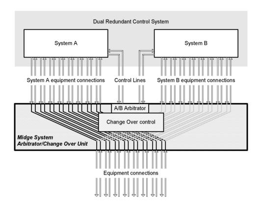
The Integrated Arbitrator and 8 Port Change Over Unit interfaces to a dual redundant control system by way of "Health" and "Force" signals from each of the control system sides. The microprocessor controlled arbitrator circuitry selects a system by analysing the systems' signals and issuing an "Online" signal to the selected side. The Change Over circuitry then connects the selected side to the attached equipment connections by way of voltage free relay contacts.
