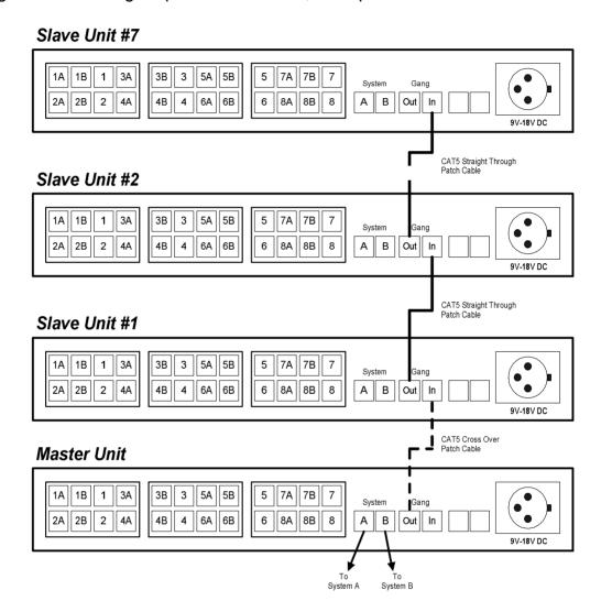
Slave mode operation is selected from via the RS232 configuration port. Slave mode has no configurable parameters.
